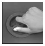
Turn the center nut on the compact spare tire cover counterclockwise to remove it. Then remove the cover.
